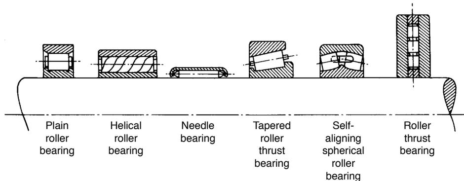
**Fig. 1-11 Types of Roller Bearings**
