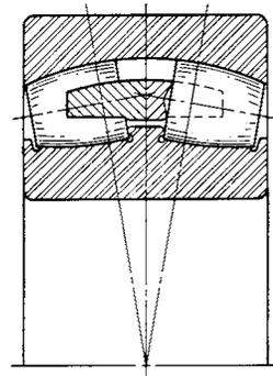
**Fig. 1-13 Self-Aligning Spherical Roller Bearing for Radial and Thrust Loads**
