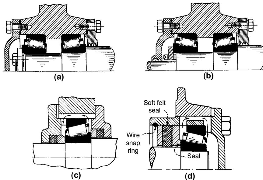
**Fig. 1-12 Details of Mounting of Roller Bearings**
